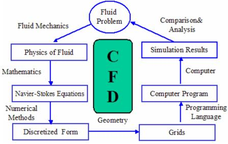
Figure 1 Process of Computational Fluid Dynamics
