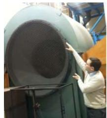
Figure 3 : The Inlet duct of the blowing fan for the wind tunnel its reasonably large.
