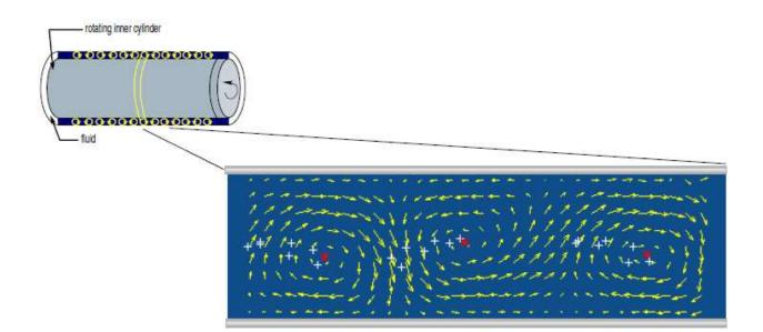
difficult to find CFD codes that can be run over the internet from any typical browser. Here we display a few results produced by such codes to indicate the wide range of problems to which CFD has already been applied, and we will briefly describe some of the potential future areas for its use. The figure in the lower left-hand corner provides a direct comparison with experimental
