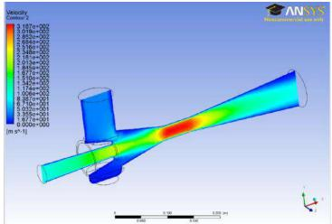
Figure 4: A throttle valve describes and internal flow example, where maximum velocity is achieved at the minimum area cross section (throat).
